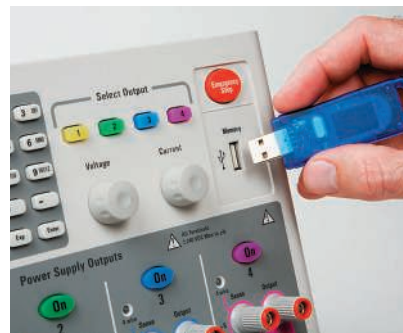
Figure 12. The N6705's front panel USB port.
